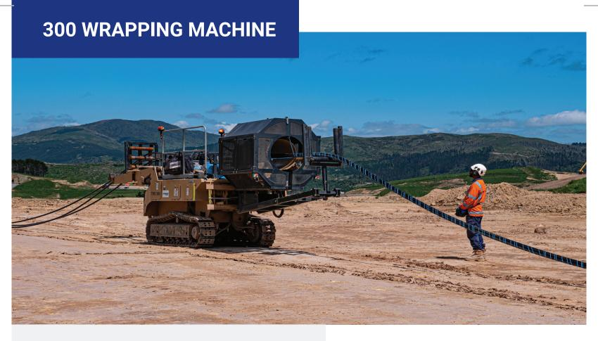
Tesmec 300 Wrapping Machine is a 6 metric ton-class machine featuring a 73 Hp (54.5kW) Tier 4 engine designed to bundle cables or HDPE ducts in trefoil. It is conceived for energy cable projects.
